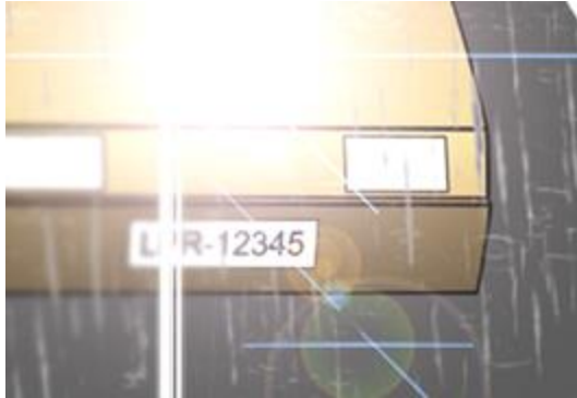
License plate image with smear because of overexposure
